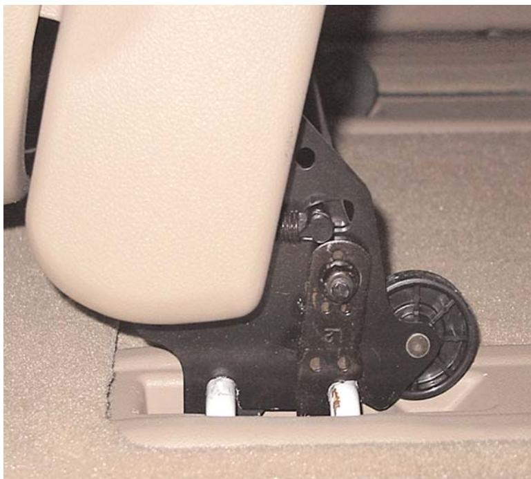
Push the seat backward until the seat fully latches to the floor. Check to see if the seat is fully latched by inspecting the seat just above the rear latches. A GREEN DOT should be visible through a small round hole. (See photo)
