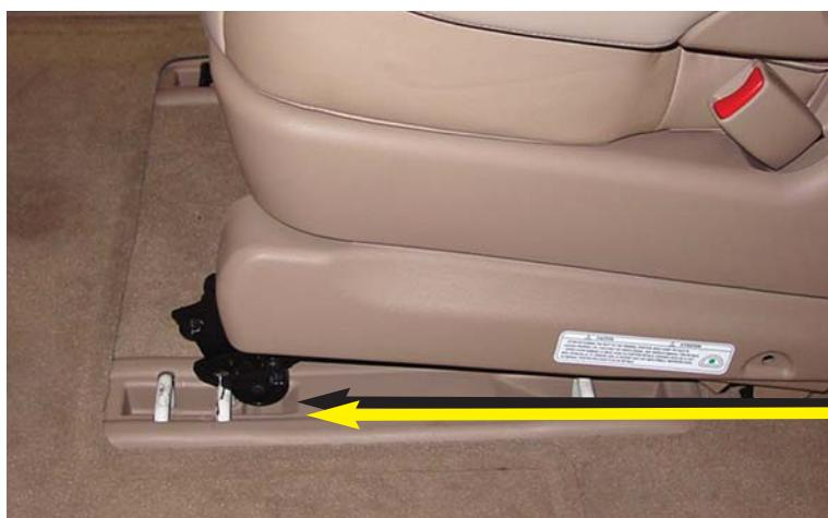
Applying light pressure to the front of the seat, grasp the rear of the seat and carefully roll it forward until the front of the seat latches to the floor. (See photo)
